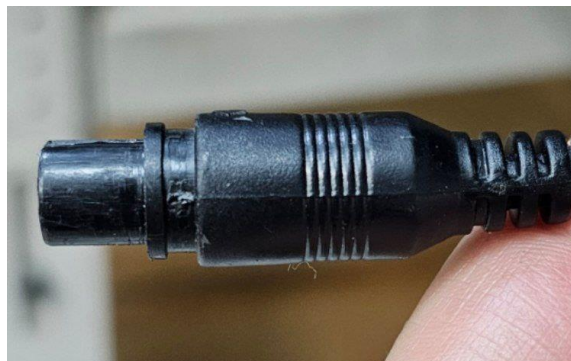
Connector for connection of GX12 (4 contacts), supply voltage 24 V
