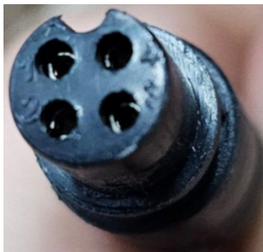
Connector for connection of GX12 (4 contacts), supply voltage 24 V
